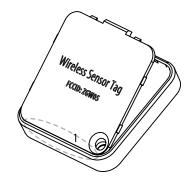
Step 3. Close the lid by pushing down where the hooks  $(2\sim4)$  are, one at a time
